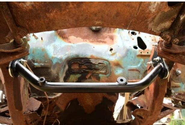
This picture shows the crossmember properly installed and ready to receive the new rack.
