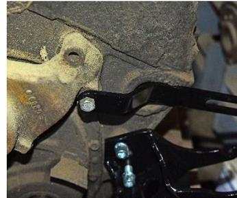
16. Bolt the new power steering pump to the brackets using the bolt holes identified in the pictures below.
