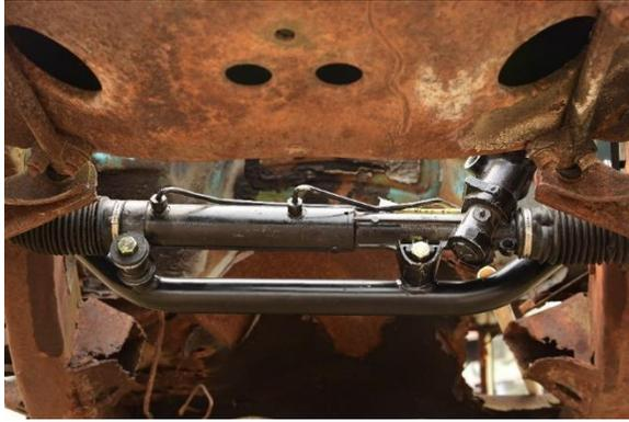
25. Install the rack to the crossmember using the supplied hardware.
