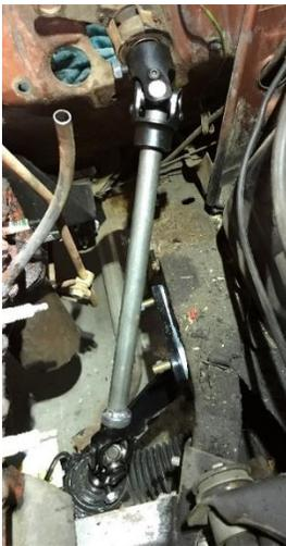
Once you are satisfied with the length/cut of the steering shaft and have installed the brass bushing in the end of the OE column (just a reminder these are not steps you need to take with most aftermarket columns) you can install the column inside the car. Hook it up to the intermediate shaft and hook up the intermediate shaft to the rack as shown in this picture.
