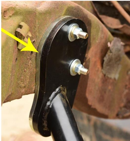
24. Install the 2 supplied bolts, nuts, and washers to secure the passenger side of the crossmember.
