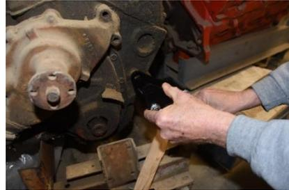
11. Install the upper adjusting bracket into the lower water pump bolt hole as shown in the picture on the previous page.
