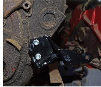
14. Reinstall the motor mount bushings and hardware and allow the engine to rest again on the new mount.
