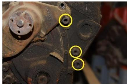
13. Bolt the lower bracket into place on the block into the lower 2 holes identified in the pictured on the previous page.
