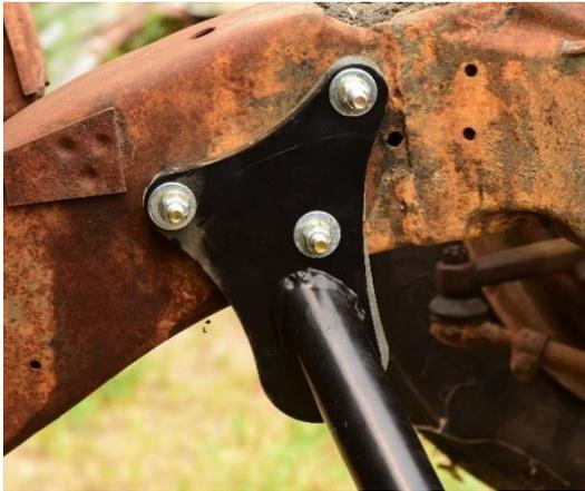
23. Install the 3 supplied bolts, nuts, and washers to secure the driver side of the crossmember.
