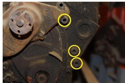
9. Ensure your lower bracket is assembled as pictured here to install properly on the block.
