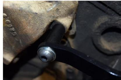
12. Bolt the new power steering pump to the brackets using the bolt holes in the pump identified in this picture.
