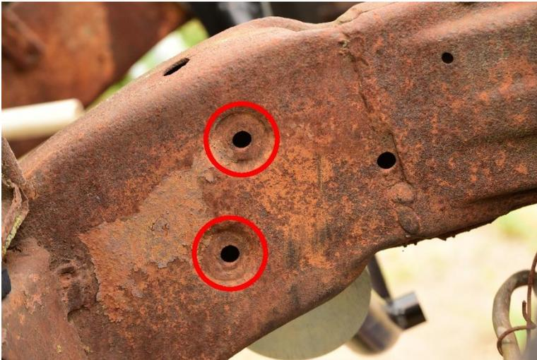
This picture shows the passenger side frame rail. These 2 holes, identified with RED circles, are the idler arm bolt holes. These 2 holes are the holes you will use to bolt the passenger side of the new rack and pinion crossmember to the frame.
